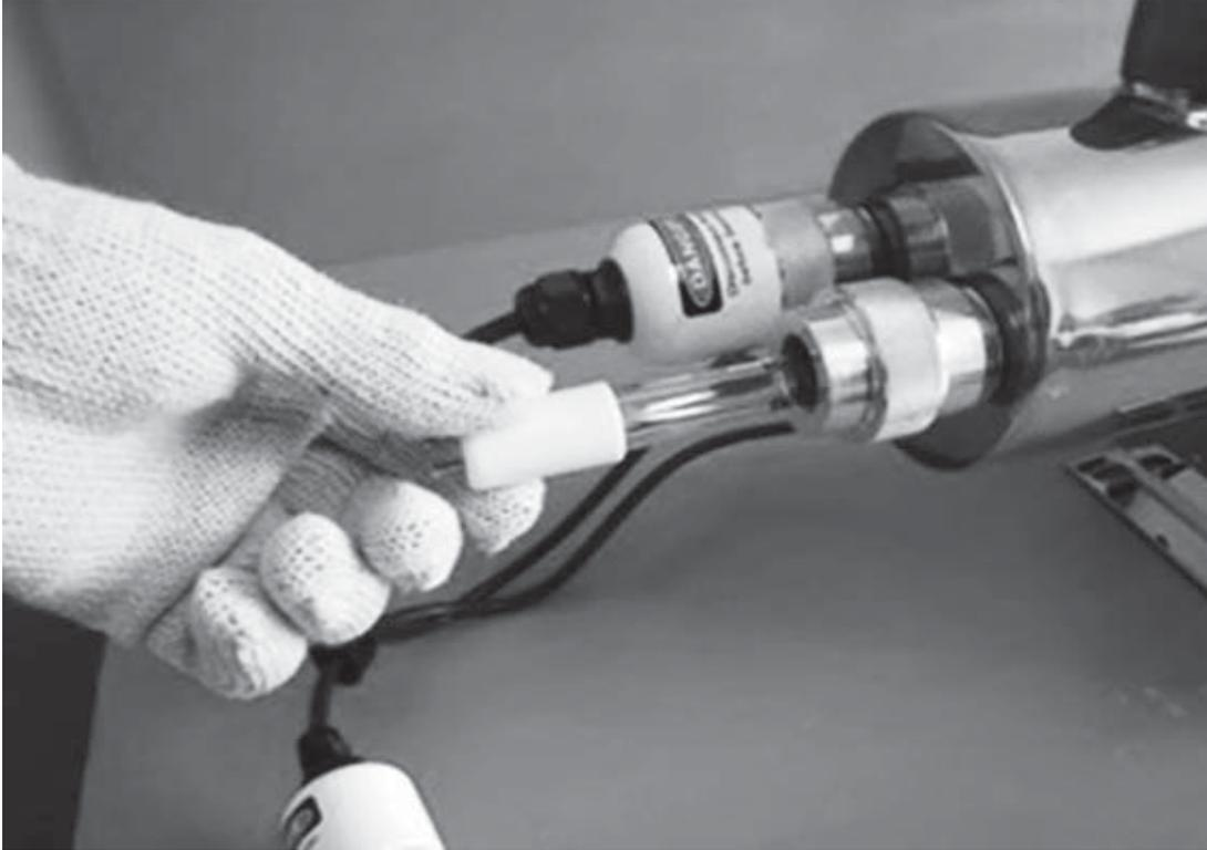
7. Follow up Lamp installation steps to reinstall new lamp.
