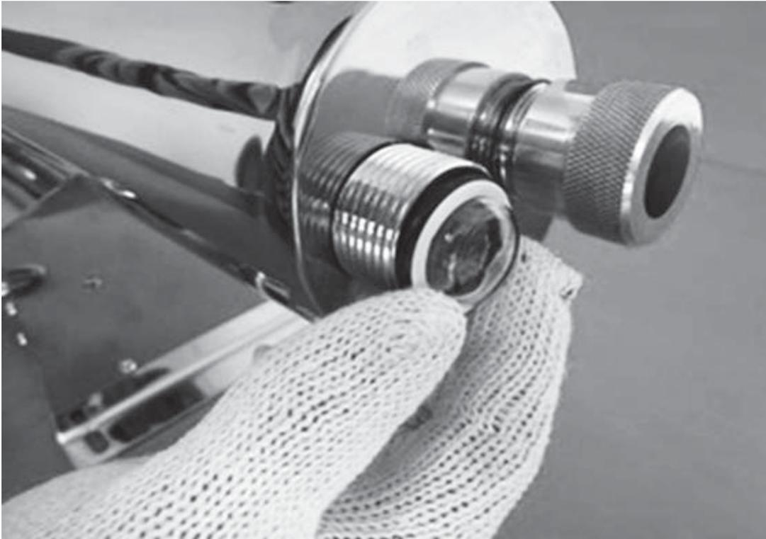
5. Reinstall Nuts on both sides of reactor chamber. Tighten nuts firmly by hand only. **DO NOT USE HAND TOOLS.** Tightening with hand tools is likely to cause quartz sleeve to break.
