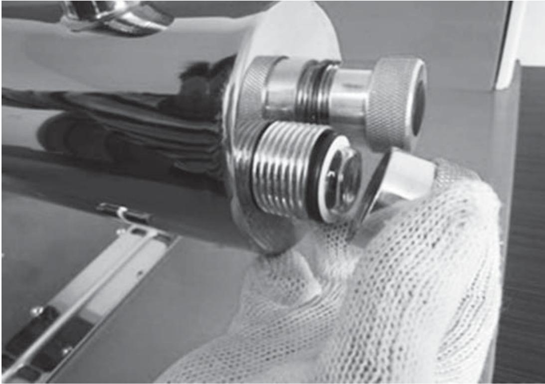
6. Slide UV Lamp into Quartz Sleeve carefully. Be sure to slide into quartz sleeve without angling.
