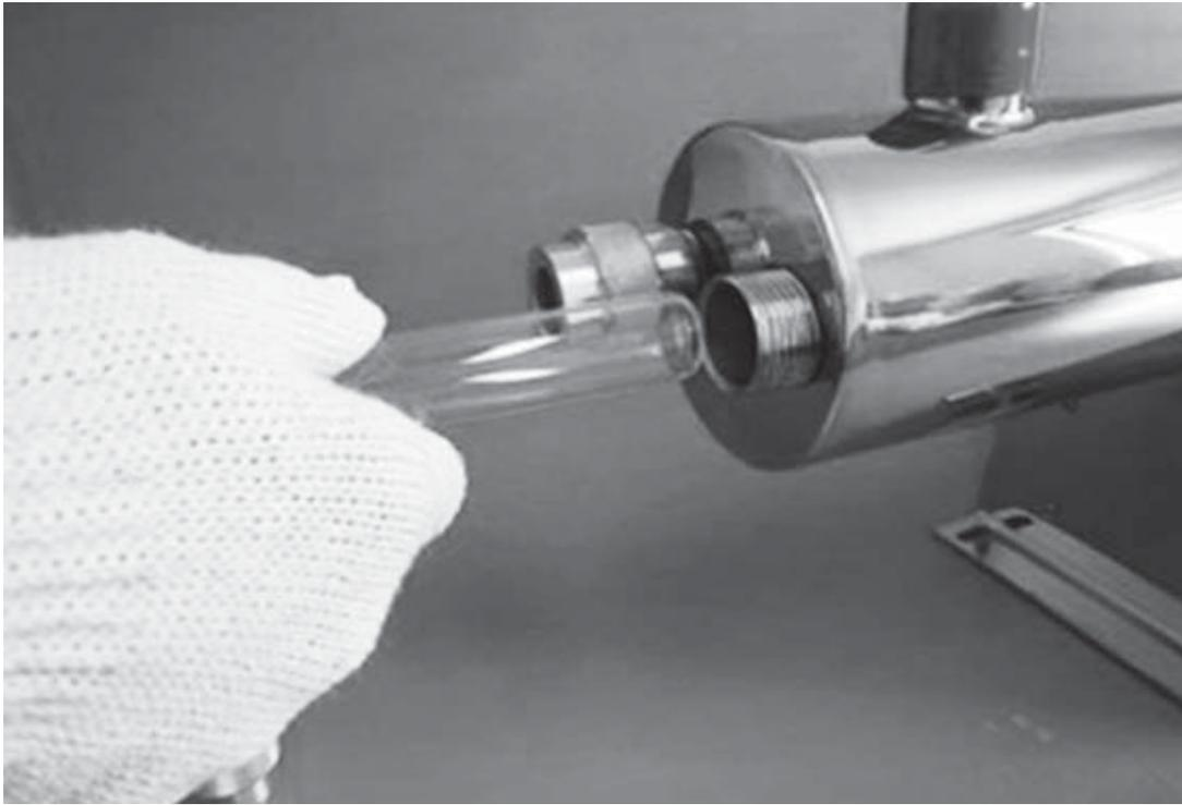
4. Install O-ring and Washer on both ends of Quartz Sleeve and Be sure O-rings are placed on quartz sleeve before Washer.
